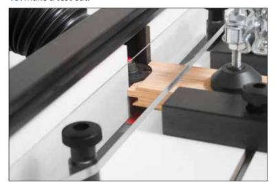
**14.** If necessary, repeat the router bit height setup process until the stile and rail mate perfectly as shown below.
